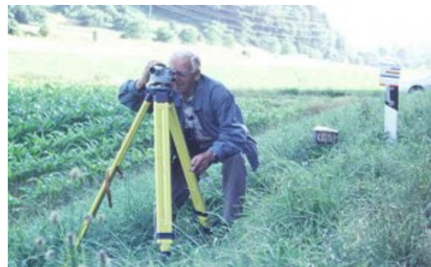
The theodolite is turned 180° and checked against the measuring post at 996 m and then the result is marked.
