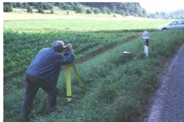
The original zero mark is set at a distance of 4 meters
